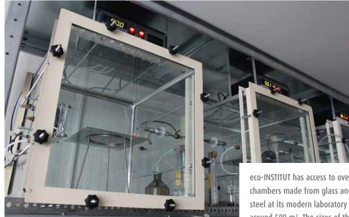
eco-INSTITUT has access to over 120 test chambers made from glass and stainless steel at its modern laboratory measuring around 500 m<sup>2</sup>. The sizes of the chambers range from 100 l to 20 m<sup>3</sup>.
